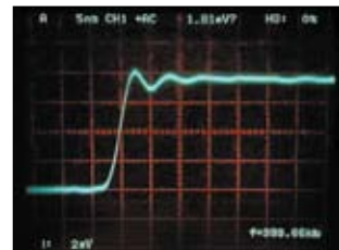
Input: 100 mAp-p (Oscilloscope bandwidth 400 MHz)
